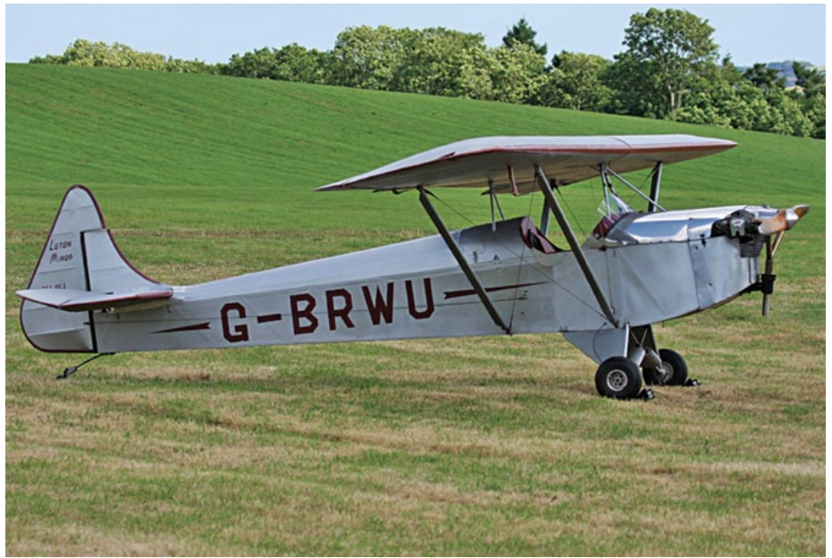
Richard also owns Luton Minor G-BRWU which is powered by a J99 Jap boxer twin. It has unfortunately been out of the air for a couple of years but will hopefully be airborne again before too long.
